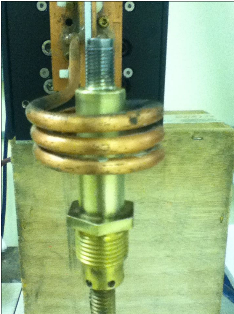
The brass tube assembly inside the induction heating coil
