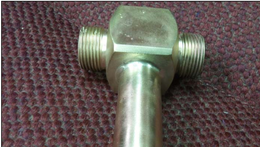
The larger assembly after being brazed and wire wheeled.
