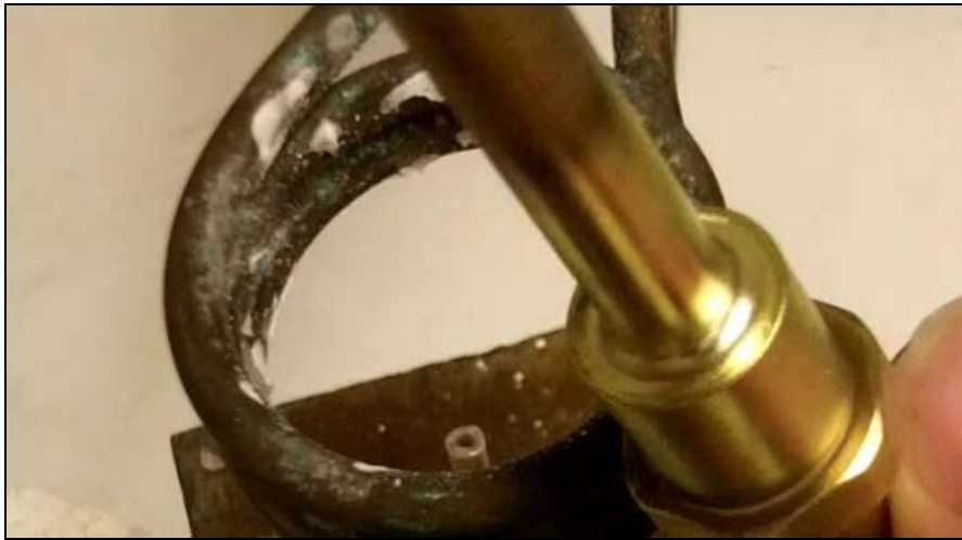
The smaller assembly after being brazed and wire wheeled
