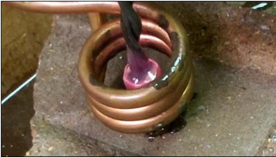
The coupler and wire being brazed together
