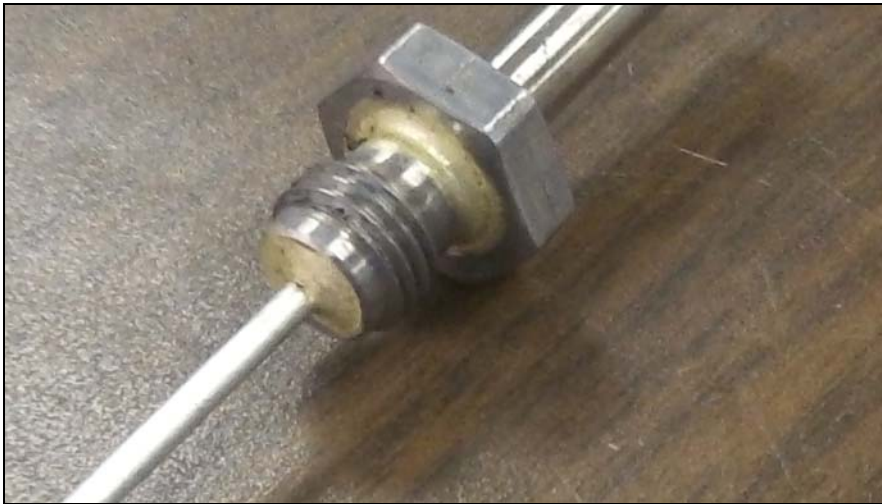
The assembly after brazing.
