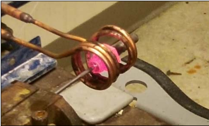
The assembly heating to temperature inside the coil. Note the gap in the coil to prevent overheating.
