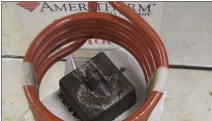
Removal of the cutter from the coupon
