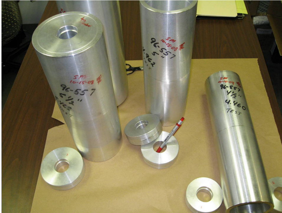
Aluminum rollers and end plugs prior to curing
