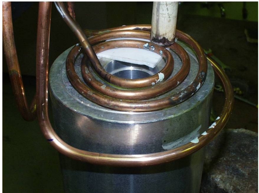
Aluminum roller and end plug assembly in coil
