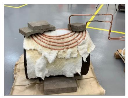
The coil is positioned on top of the steel tube, and the cinder blocks prevent levitation of the coil.
