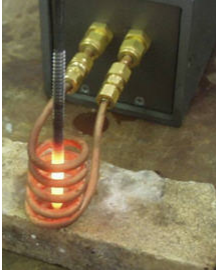
Roofing screw in coil hardening a 2" zone
