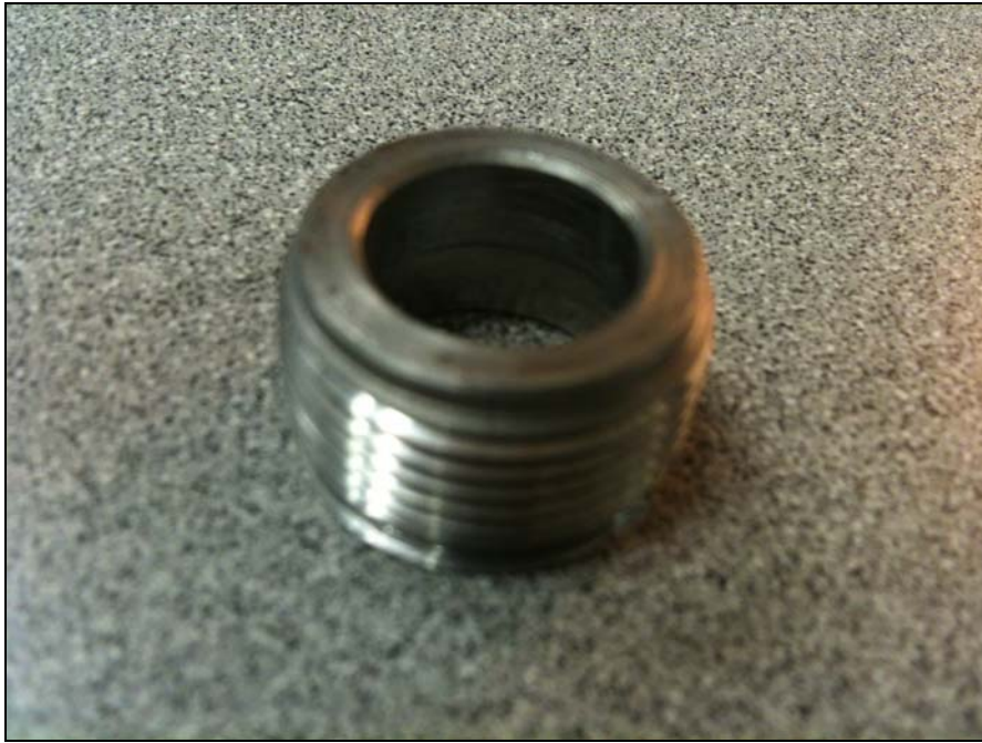
The steel fitting that is being heated for this hardening application
