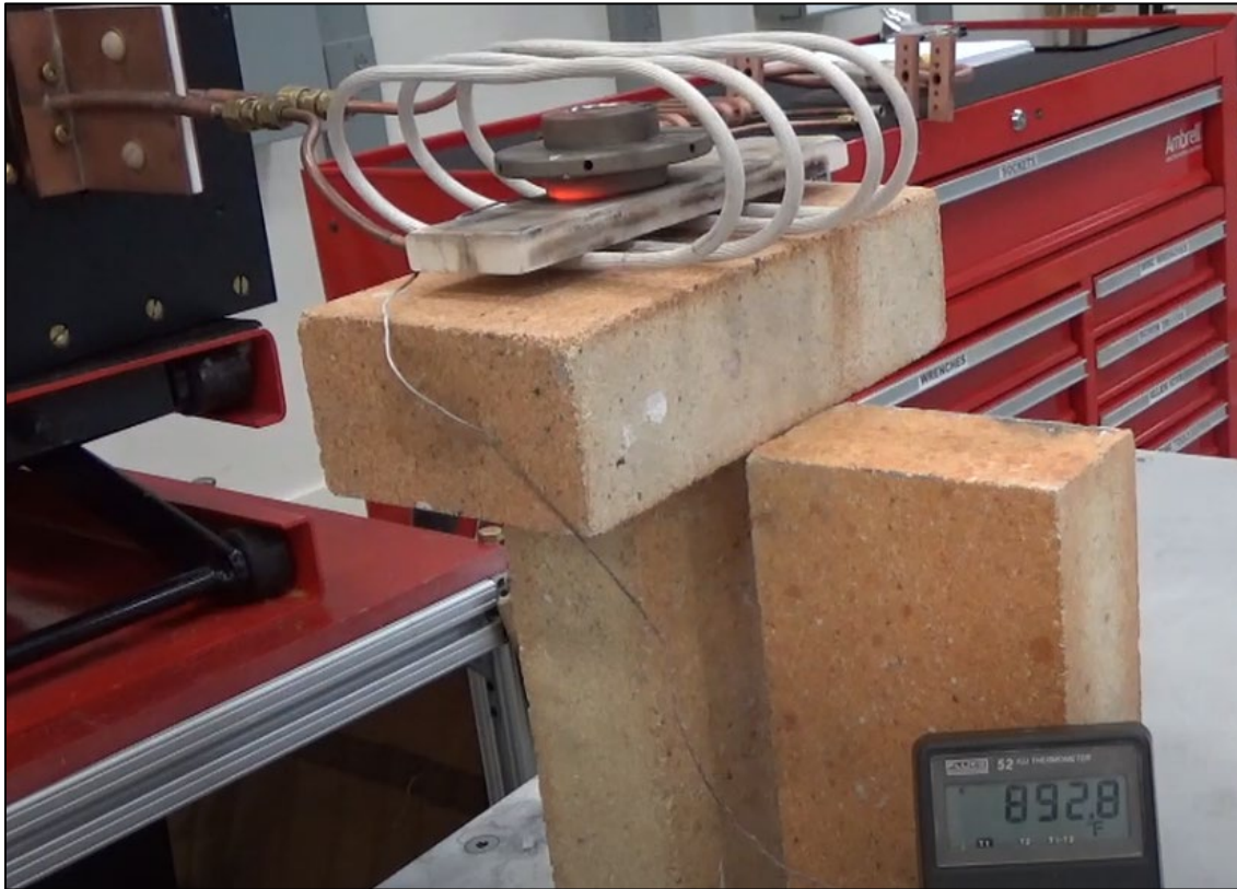
The part inside the oval coil during heating.
