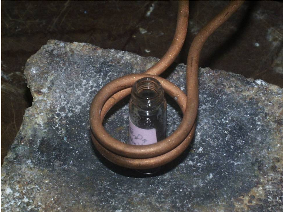
Glass vial with magnetic iron oxide in coil heating
