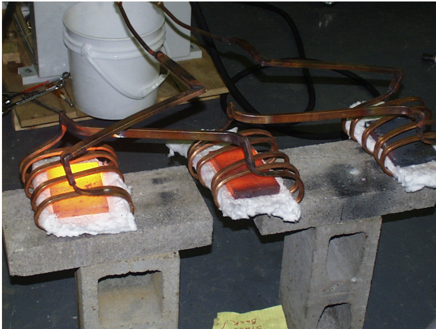
Steel plates being heated with a three position, multi-turn helical coil
