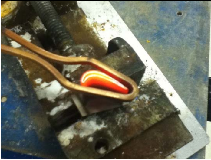
The small turbine blade being heated within the induction heating coil
