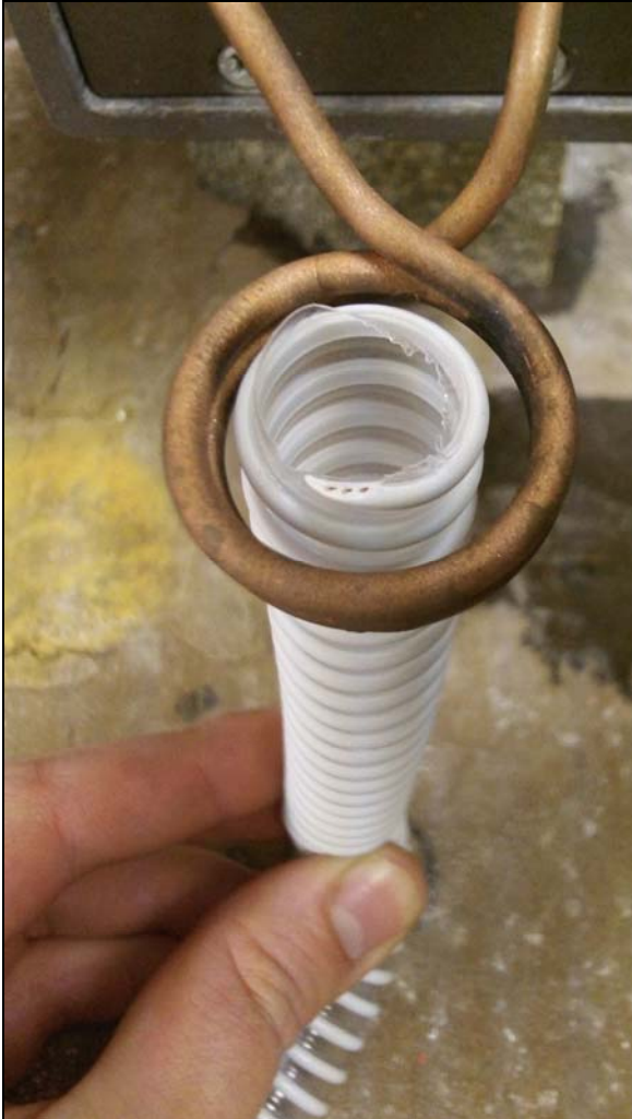
The coiled, plastic coated copper wire inside the induction heating coil
