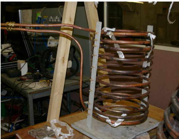
Helical coil used to heat crucible
