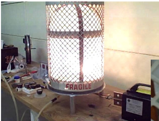
Heating of crucible under Pyrex jar with the nitrogen flowing in from underneath
