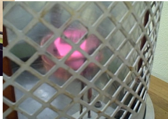
Heating of crucible under Pyrex jar with the nitrogen flowing in from underneath
