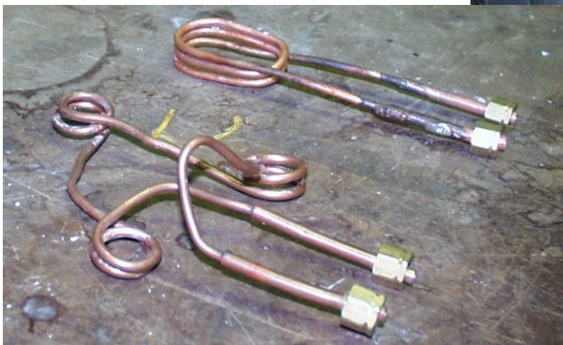
Oblong coil for heating two inserts in close proximity and three place coil for heating three inserts
