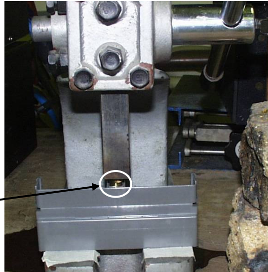
Pressing brass bushing into wire connector
