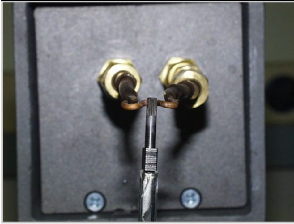
The steel shaft during heating.
