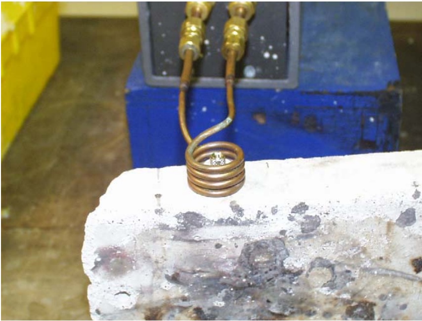
The small steel insert inside the coil with a threaded brass rod inside it.
