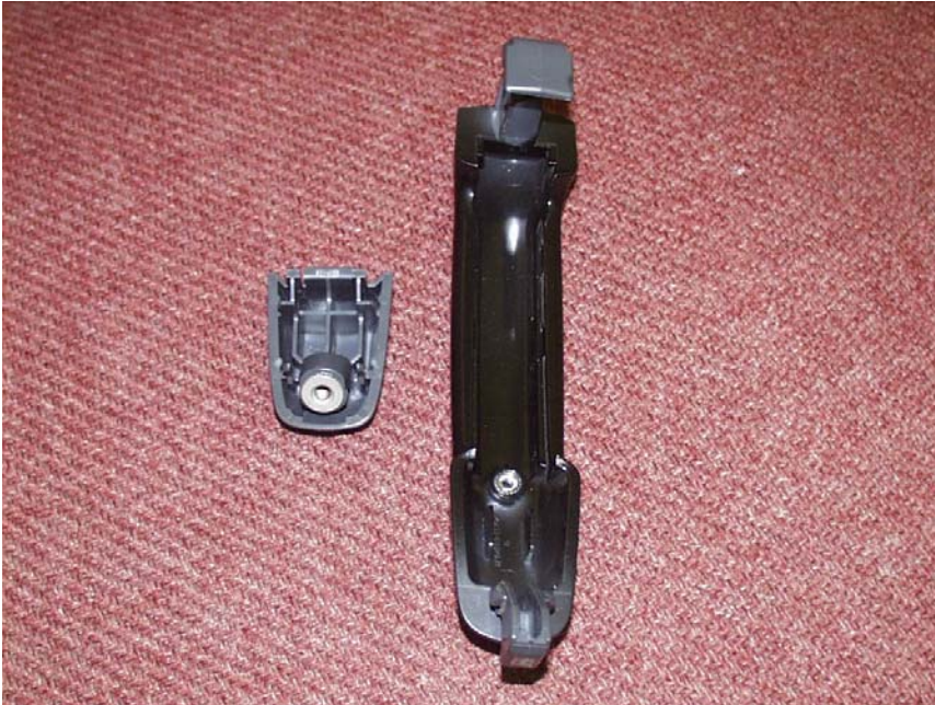
The small and large steel inserts inside their respective mating plastic pieces.
