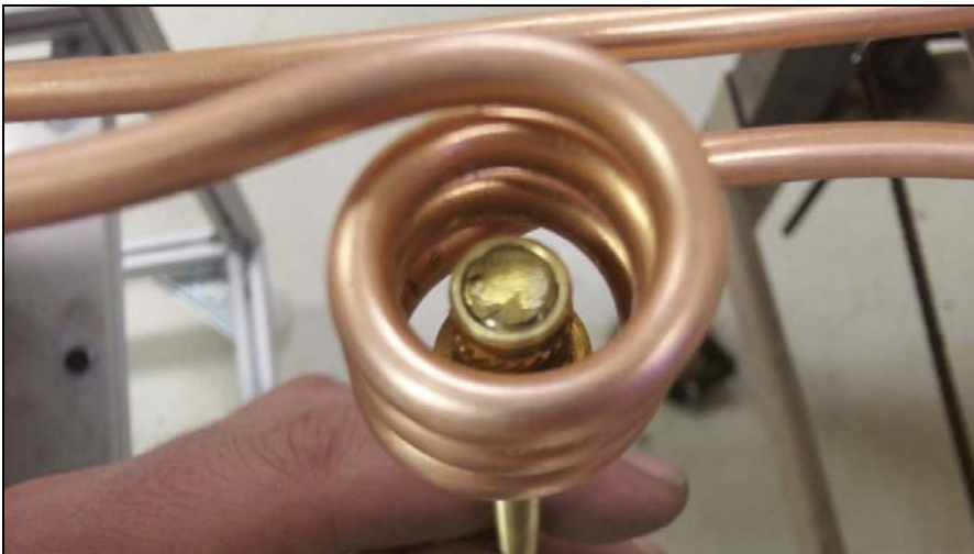
The part inside the helical induction heating coil.
