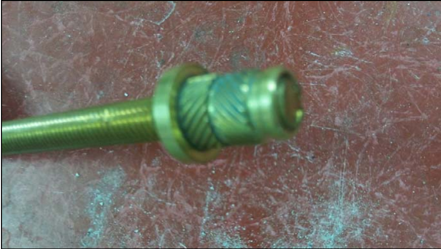
The brass insert that requires heating.
