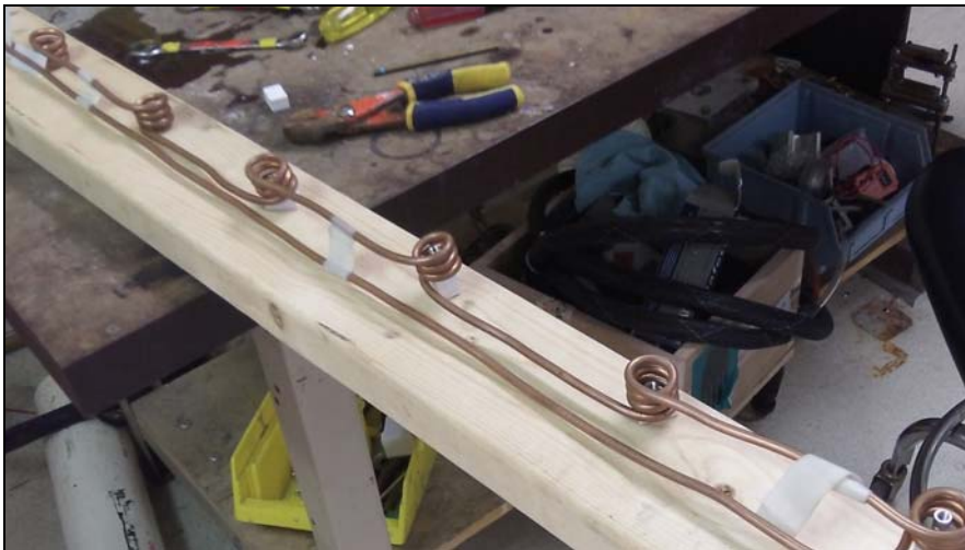
The six position coil with inserts placed inside each position
