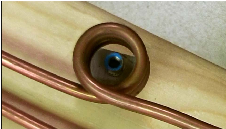
An insert with temperature indicating paint applied inside one of the coil positions
