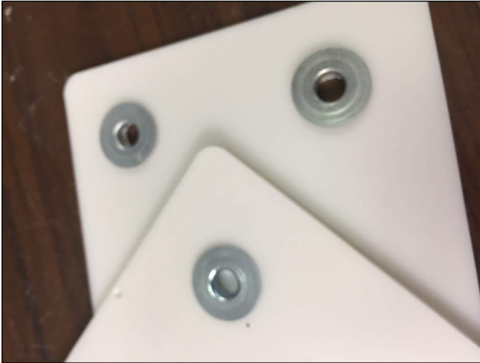
The client's assembly after conclusion of the metal-to-plastic insertion process.
