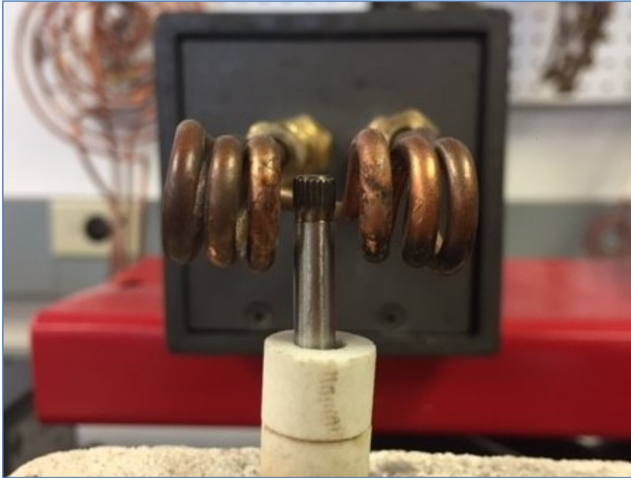
The magnetic steel tube set-up inside the multiple-turn split helical coil.
