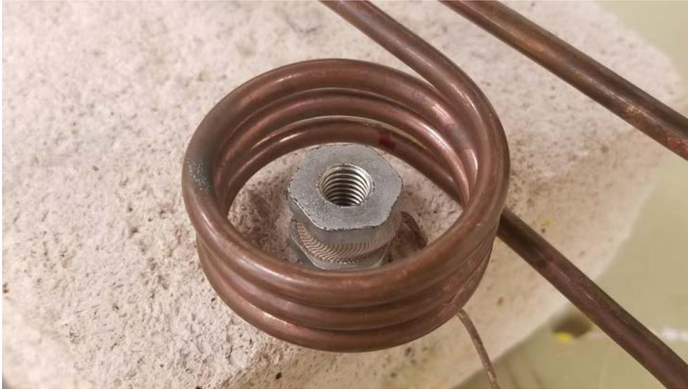
The steel insert inside the coil with a thermocouple attached.
