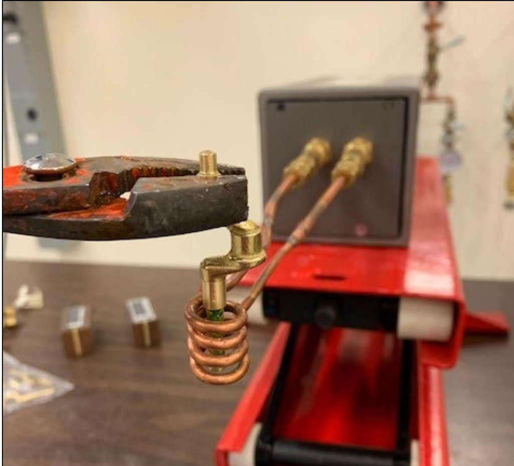
The brass shaft inside the induction coil.
