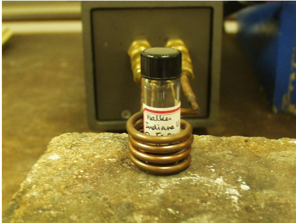
Vial of magnetite \text{Fe}_3\text{O}_4 in coil
