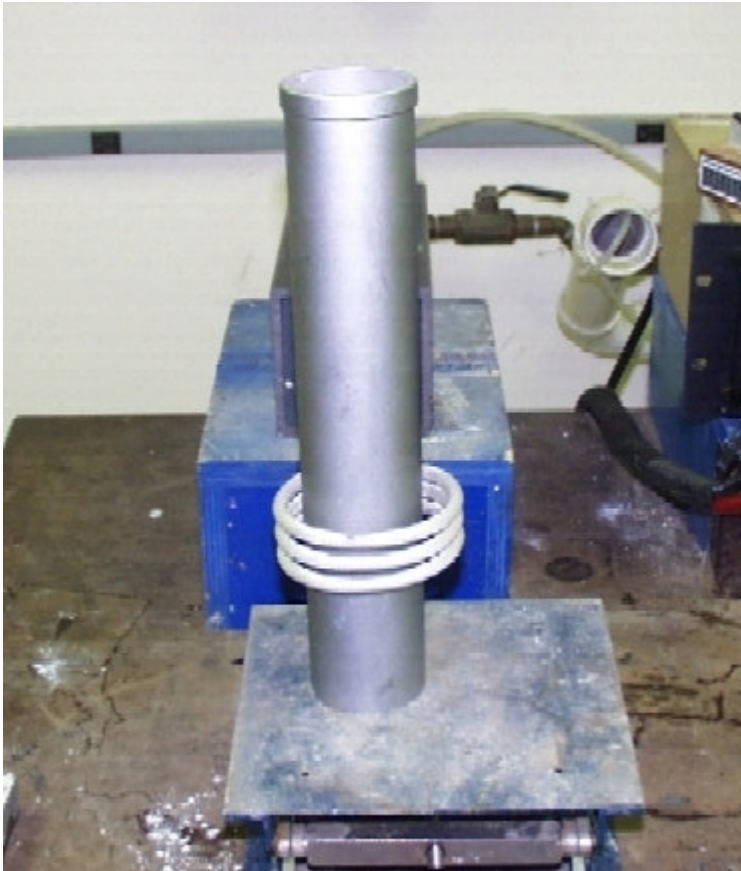
Roller placed into induction heating coil
