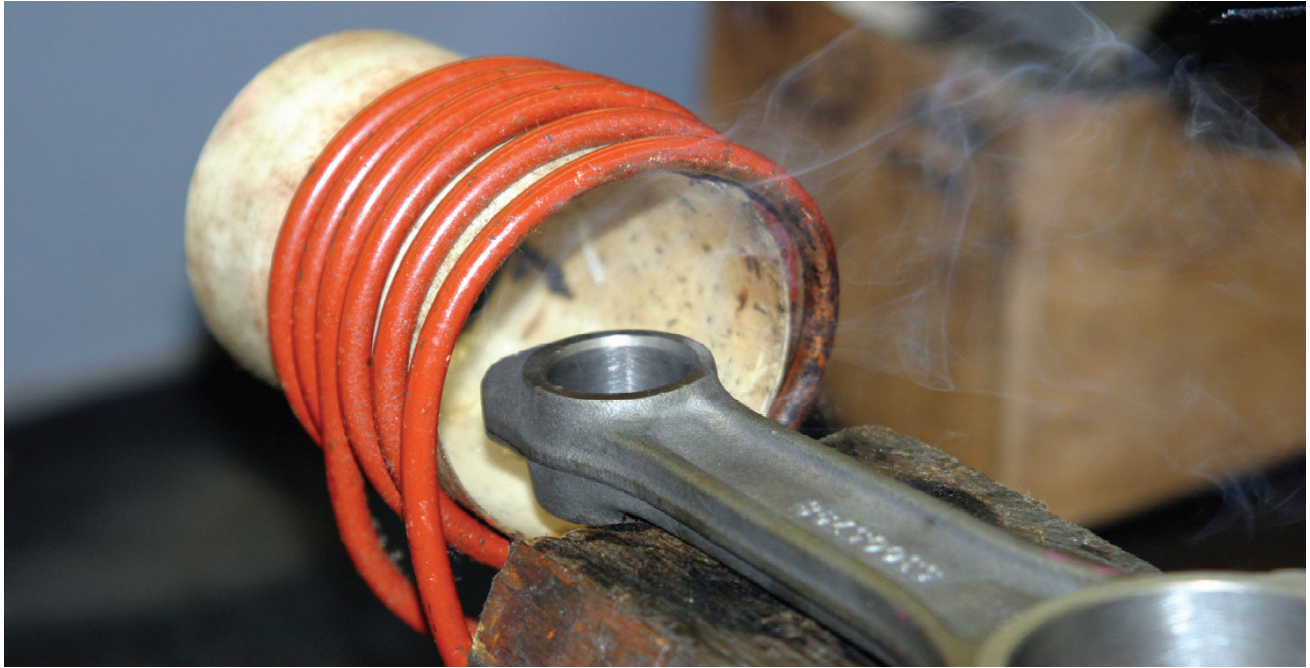
Coil is perpendicular to the axis of the bore when heating the knuckle
