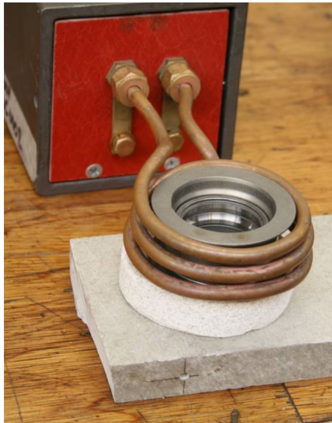
Pulley in coil prior to heating
