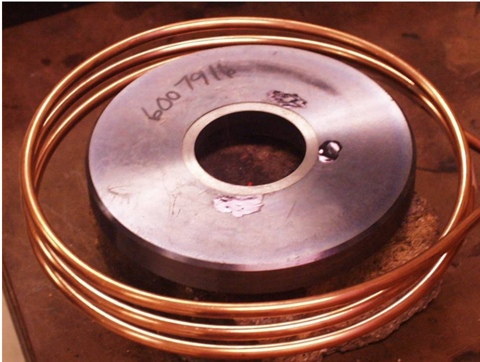
Steel valve seat with carbide ring inserted
