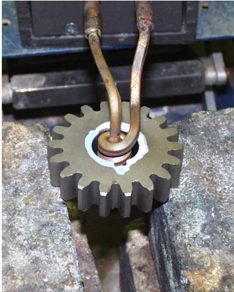
Coil inserted into gear bore prior to heating. 400 °F (204 °C) (Pink) and 500 °F (260 °C) (Blue) temperature indicating paint is used.
