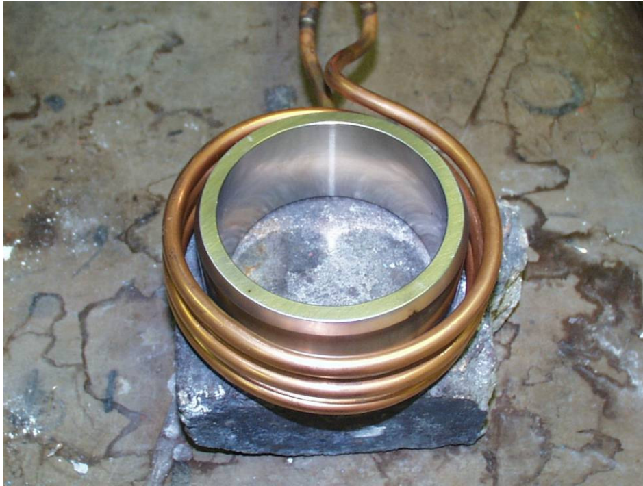
Stainless steel sleeve heating in coil prior to shrink fit application
