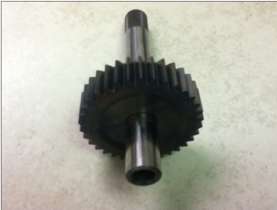
The gear and shaft after shrink fitting
