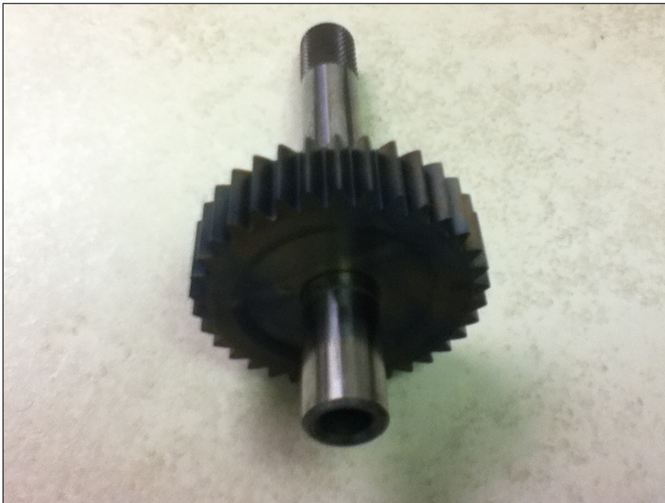
The gear and shaft after shrink fitting
