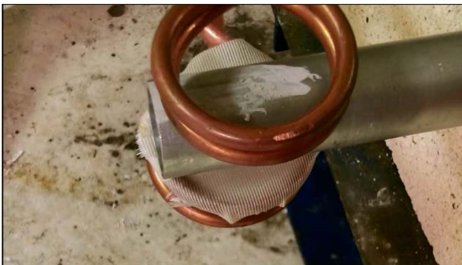
The part inside the coil with temperature indicating paint applied
