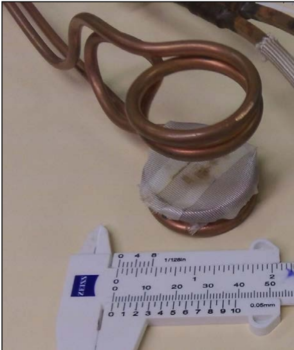
The split helical coil enabled easy loading
