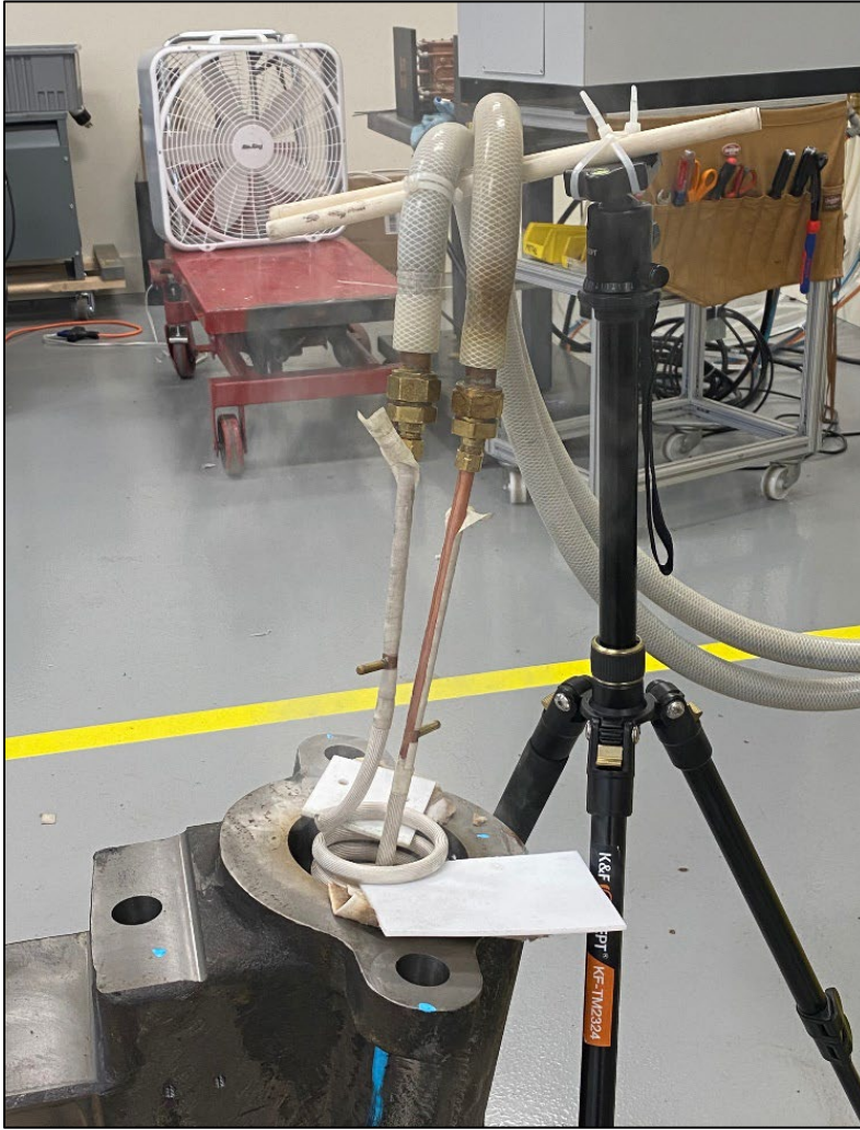
The internal helical coil designed by THE LAB at Ambrell.
