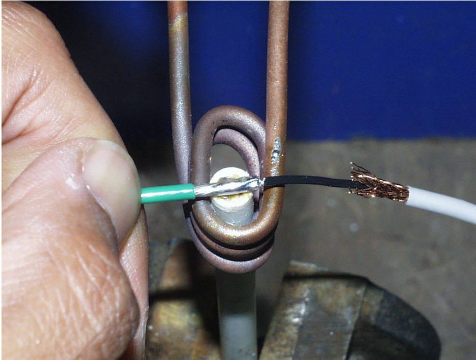
Soldering of a center conductor
