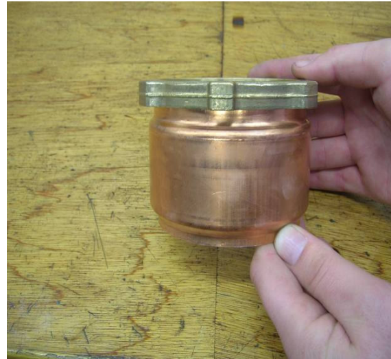
Brass ring and copper piece that will be soldered together for the 1 st step
