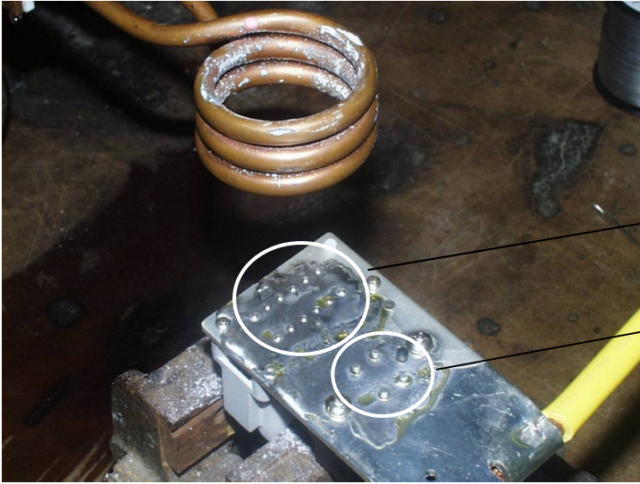
Ground plate in place for soldering of connectors
