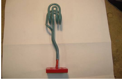
Two turn channel coil used for soldering application
