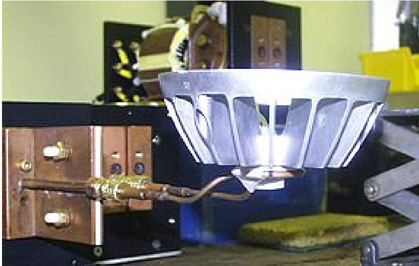
Aluminum spotlight housing placed on the coil for heating
