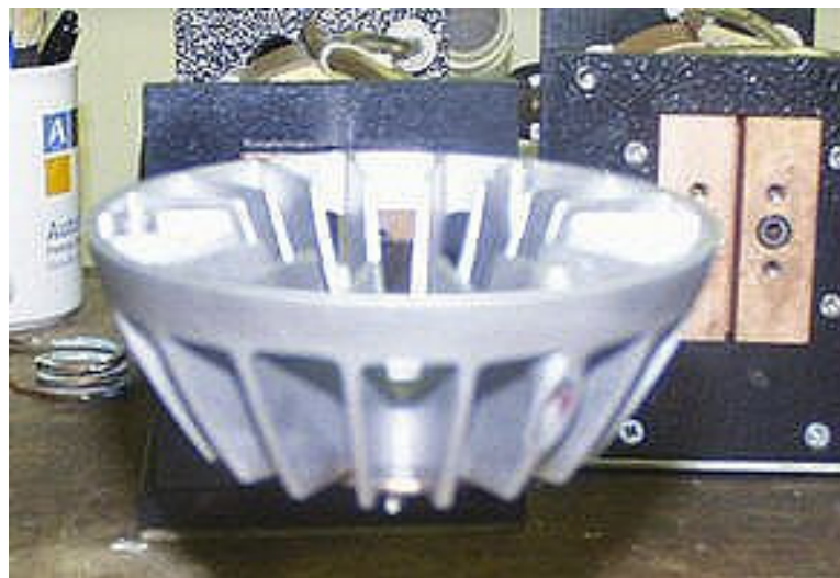
Aluminum spotlight housing placed on the coil for heating
