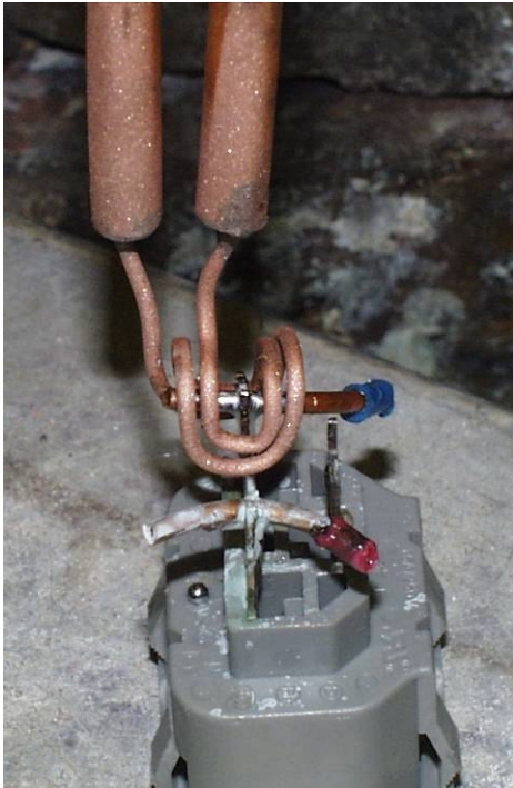
Coil in place for soldering copper wire to connector tab
