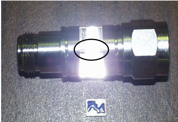
Silver dipped housing and copper chip, circle shows location of brass connector rings
