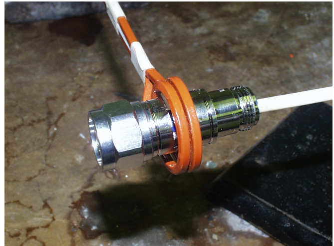
Assembly in coil for soldering application
