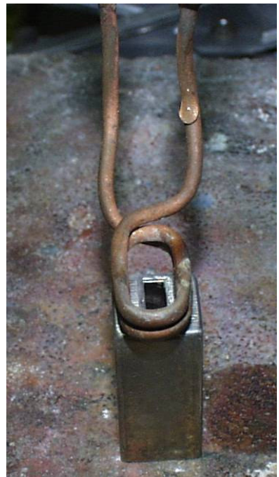
Three of the four housings heated in the same coil
