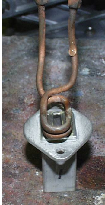
Three of the four housings heated in the same coil
