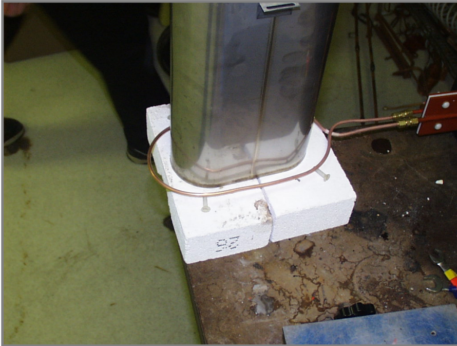
Canister is staged within single-turn coil; solder flows in the cavity formed with the steel end-plate.
