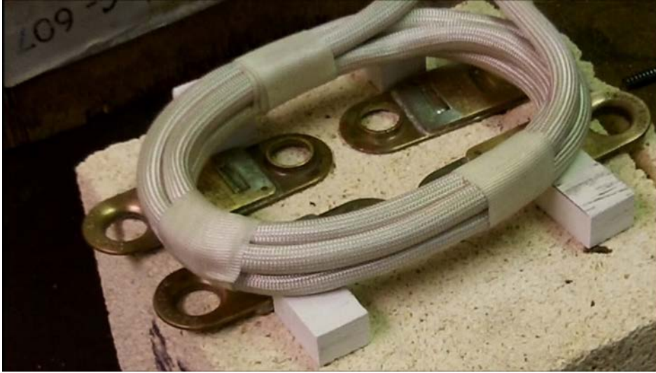
Four copper strips being heated concurrently with an induction coil.
