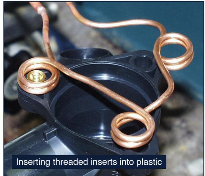
Inserting threaded inserts into plastic
